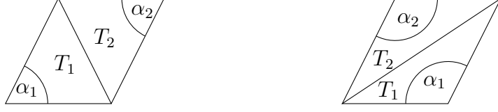
FIGURE 1. Illustration of the angle condition with notation from Definition 9. Left: configuration satisfying the angle condition. Right: configuration not satisfying the angle condition.
