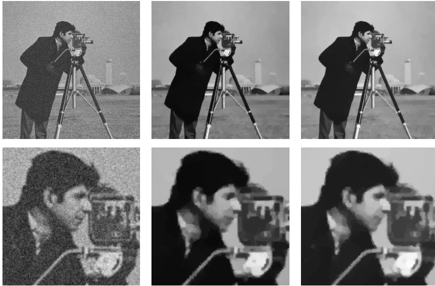
FIGURE 8. “ROF” denoising example. Left: noisy image. Middle, denoised with \varphi(\nu) = |\nu_1| + |\nu_2| . Right: with the effective tension computed for T = 4 .
