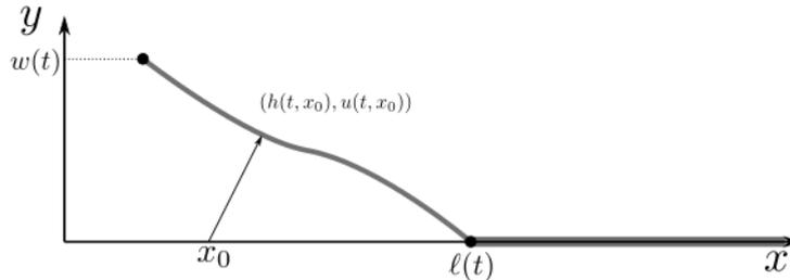
FIGURE 1. The deformation of the film at time  $t$  is represented by the displacement  $(x_0, 0) \mapsto (x_0 + h(t, x_0), u(t, x_0))$ . The function  $w(t)$  is the vertical loading, while  $\ell(t)$  is the debonding front.
