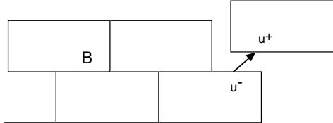
Figure 1. Admissible deformation for a brick wall
