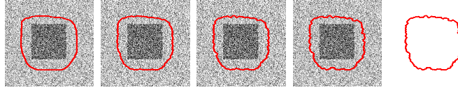
Figure 4: H^0 gradient descent flow of Chan–Vese energy, to segment a noisy square
