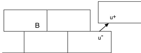
Figure 1. Admissible deformation for a brick wall
