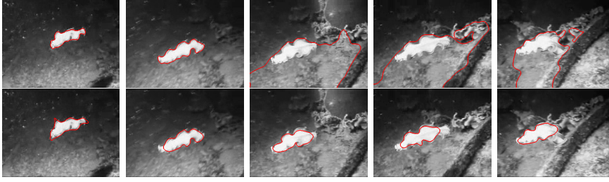
Figure 4. Tracking of a sea creature using a covariance prior from the initial frame. The top row shows the tracking using a simple Chan-Vese detection energy with Sobolev active contours. The bottom row shows the result when adding a simple covariance prior obtained from the initial frame, which can only be optimized with Sobolev active contours.
