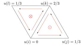
Figure 5. Discrete Burgers Circuit: According to the definition of  $\alpha_u$ , the discrete circulation of u along the edges of the triangle (i, j, k) equals 1 and along the edges of the triangle (i, k, l) equals -1.
